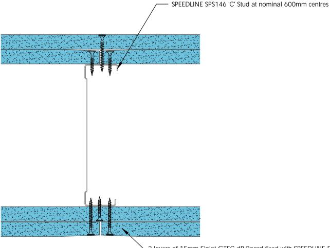
2 layers of 15mm Siniat GTEC dB Board fixed with SPEEDLINE Drywall Screws at 300mm centres (200mm centres at external angles). Ref to table for fixing length.
